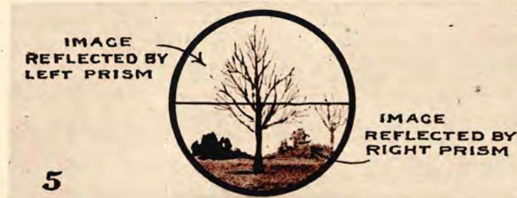
FIG. 5.—WITH THE UPPER SECTION SEEN THROUGH THE LEFT-HAND TELESCOPE AND THE LOWER THROUGH THE RIGHT-HAND: A VIEW THROUGH A ONE-MAN RANGE-FINDER.
